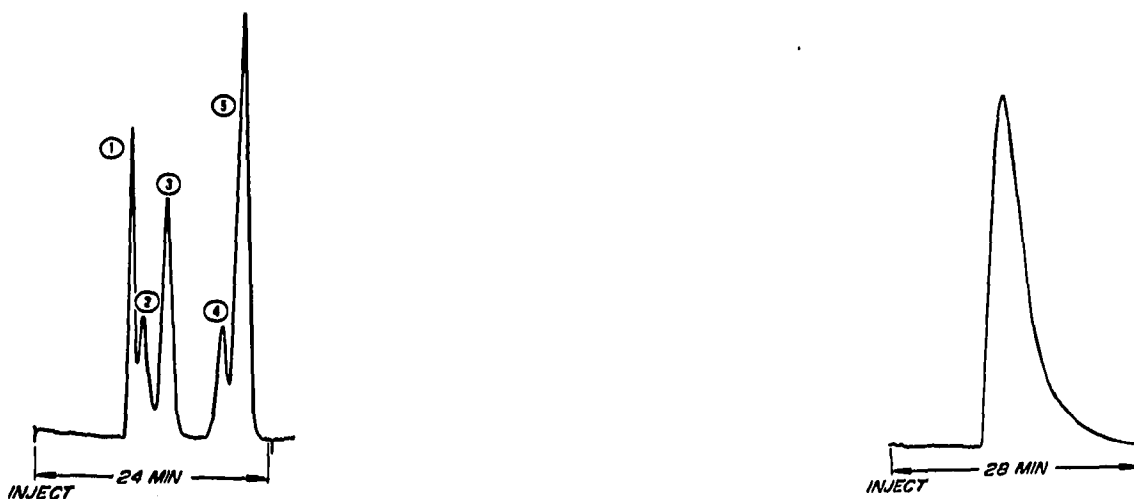
Fig. 4. Molecular-weight-distribution calibration run on Vit-X. Sample size, 3 \mu l, 10 \mu g/ \mu l; column, 2 m \times 2.6 mm; packing, 1 m Vit-X-1195, 1 m Vit-X-15300; solvent, tetrahydrofuran; flow-rate, 0.5 ml/min; detector, UV; sensitivity, 0.05 \times 1. Peaks (polystyrene): (1) M_w = 2,610,000 ; (2) M_w = 498,000 ; (3) M_w = 200,000 ; (4) M_w = 20,800 ; (5) M_w = 4000 and 2100.
